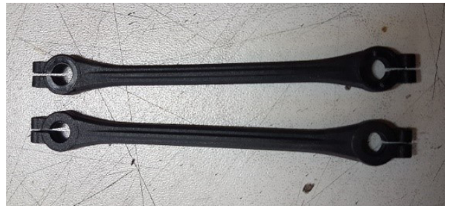
Fig 4. Note the shiny side of the side link at the top of the picture – make sure the pivot ball is installed from this side.
