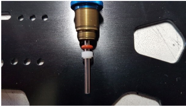
Fig 1. Note the direction of the shoulder on the rod guide.
