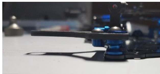
Fig 10. Note the 0.5mm spacer above the arm mounting standoff rather than below.
