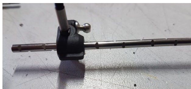
Fig 8. Run an arm reamer through the hub once the axle has been installed.
